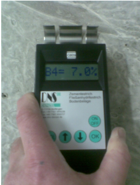
Picture 1: Control measurement on the surface of the concrete layer after 72 hours of hardening.
